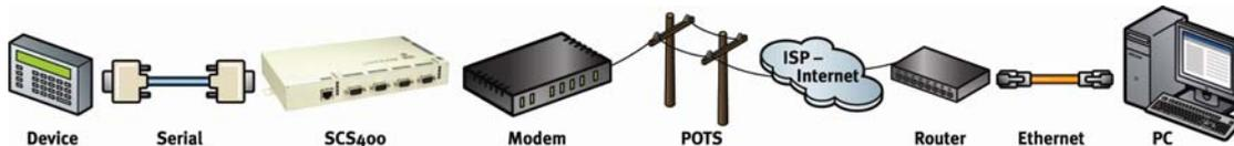
In another such scenario, the SCS400 is dialed by the client (either dial-in or dial-back). This same physical setup can be used to make a modem emulation session on the serial port of the SCS400 and trigger it to dial the host using a routing table. The layout for this would be:
