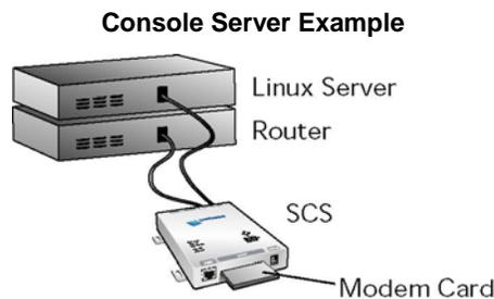
Once you have completed the physical connections, you can establish an SSH or Telnet connection to the SCS's IP address and the socket number of the desired port.
