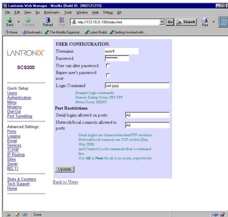
2. To configure an external serial modem, attach the modem to one of the serial ports and follow these steps:
