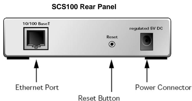
**Note:** The Reset button returns the SCS to its factory default configuration when you press and hold it during the power-up and boot process. Resetting to factory default will enable DHCP.
