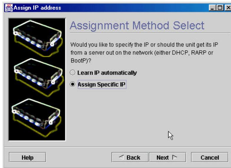
4. Select **Assign Specific IP** and click **Next**. The Assign address – IP Settings window displays.
