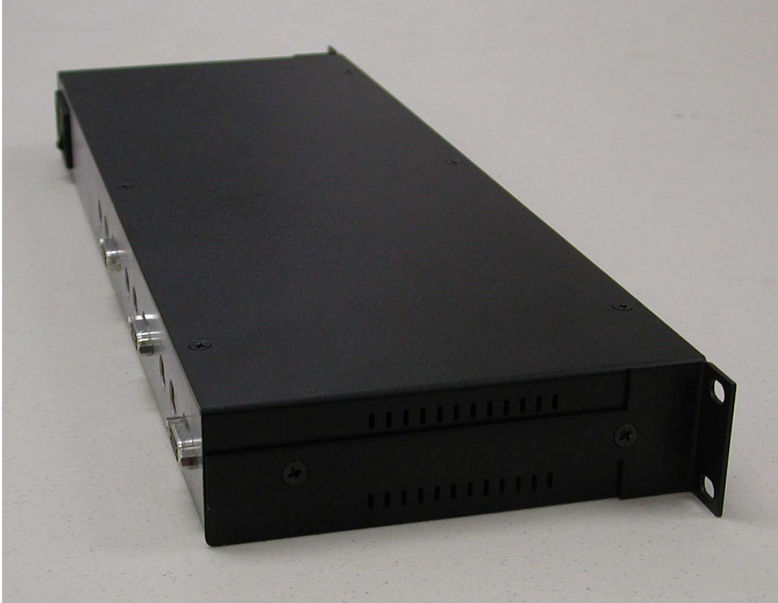
KVM 2-Port, Side View, showing removable Rack Mount bracket
