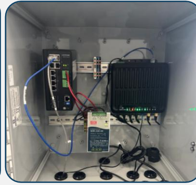
Weatherproof IP-rated enclosure with POE switch and 5G connectivity.
