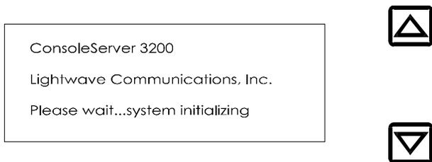
After the ConsoleServer 3200 has gone through the initialization phase, the terminal connection list will automatically be displayed. To display the next panel in a function, press the down arrow on the ConsoleServer 3200. To display the previous panel, press the up arrow.
