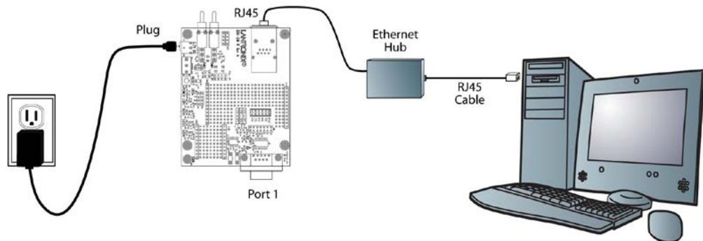
2. Select the appropriate power plug adaptor for your geographical location. Insert it into the slot on the Universal Power Supply; then plug the power supply into an outlet.
