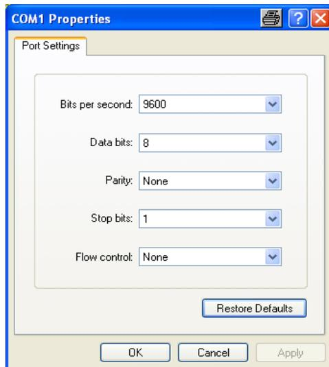
The COM Port is setup for communication. Refer to either the *XPort Pro User Guide* or the *XPort User Guide* for information on configuring your XPort device using the serial method.
