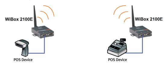
Figure 2-4. Direct WiBox 2100E-to-WiBox 2100E Connection
