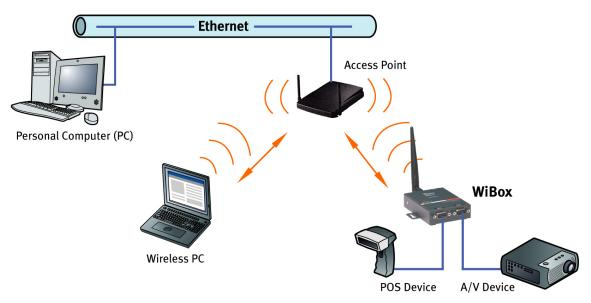
A PC connected to an AP via an Ethernet connection and a PC with a wireless connection to the AP LAN access the WiBox 2100E as though they are connected to it directly. The combination of the WiBox 2100E, a PC, and the Lantronix Redirector software allows the PC to communicate directly to the WiBox 2100E's serial devices, providing wireless serial tunneling.
