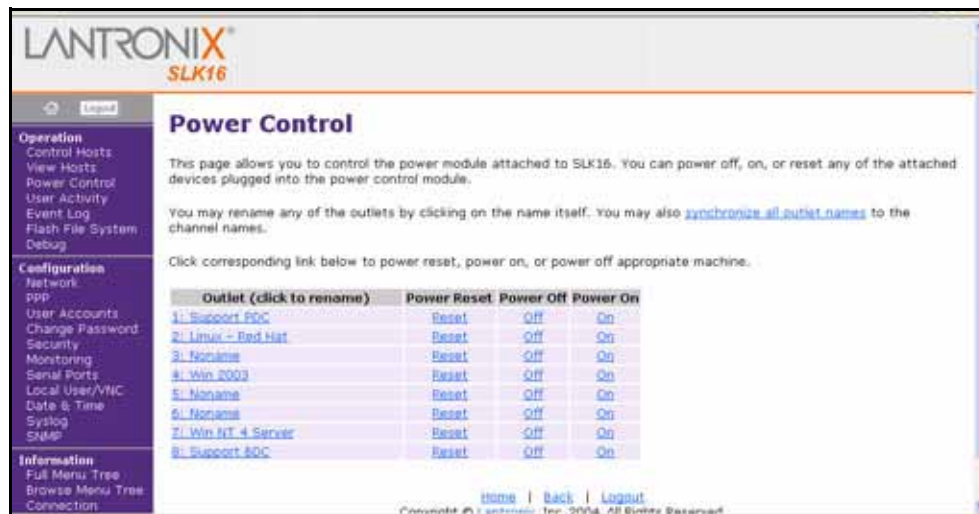
Figure 4-6. Power Control with an Optional SLP Remote Power Manager
