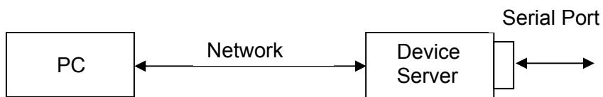
The purpose of the encryption DLL is to provide a developer with the capability of sending and receiving encrypted data between a Device Server over a network. Only Device Servers, such as the Lantronix SDS1100, SDS2100, or WiPort WPA, which have the capability to process encrypted data, can participate in this communication. These Device Servers can send and receive encrypted data using AES encryption at 128, 192, and 256 bits.
