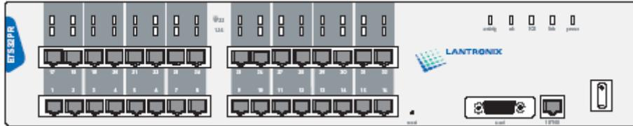
**Note:** The first RJ45 port is also the serial console port. Use it as a method for the initial setup or troubleshooting.
