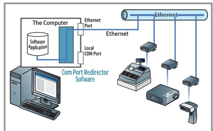
Conversely, data sent from the networked equipment to the serial port of the device server is transmitted back to the application software on the PC via Ethernet. Com Port Redirector receives the data and presents it to the control application as if it came from a COM port via a local serial connection.
