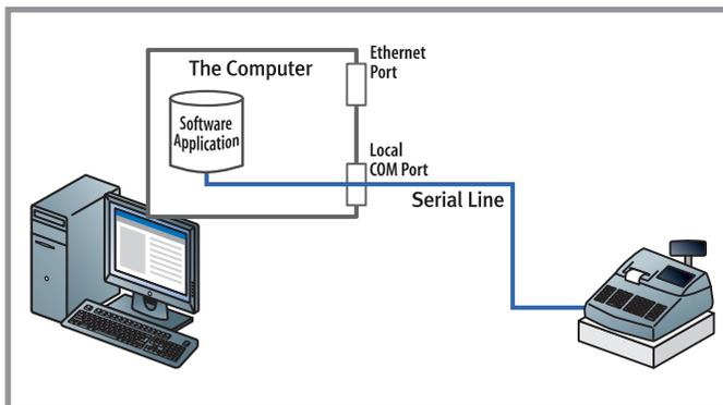
As long as the attached device is within the limited distance reach of the PC, this works great. But, the moment the device is placed on an Ethernet network and direct serial connection is broken, the ability of the application software to communicate with the device is lost. That's where Com Port Redirector comes in.
