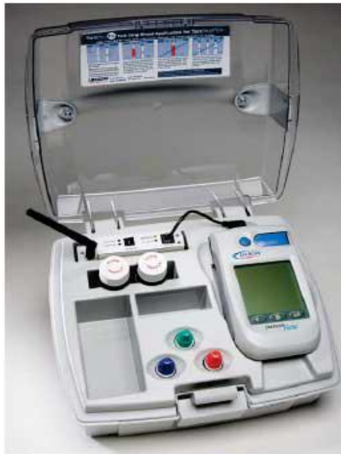
A custom battery-powered version of the WiBox™ is integrated into the LifeScan OneTouch® DataLink® Unit.
