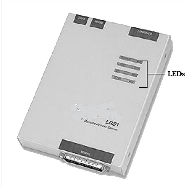
The first LED is a power indicator, and should remain green while the LRS is plugged in. The second is a network link indicator, and should remain green when the LRS is properly connected to the network. Throughout the manual, these LEDs will be referred to as the Power and Link LEDs.
