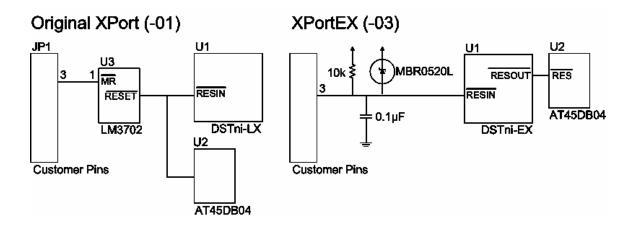
**Note:** The LM3702 MR in the XPort (-01) has an internal pull-up resistor of approximately 56k  $\Omega$ .
