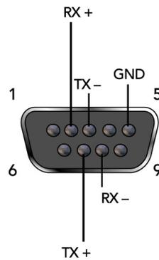
Figure 2-7. RS-485 2-Wire Pinouts
