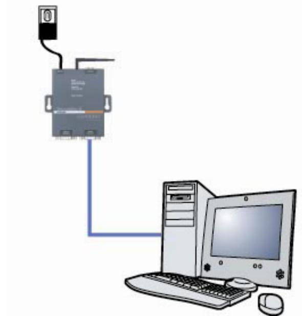
1. Connect one end of the supplied DB9F – DB9F null modem serial cable to the WiBox 2100E's serial port 1.
