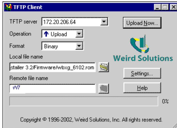
After the firmware has been loaded and stored, which takes approximately 8 seconds, the unit performs a power reset.
