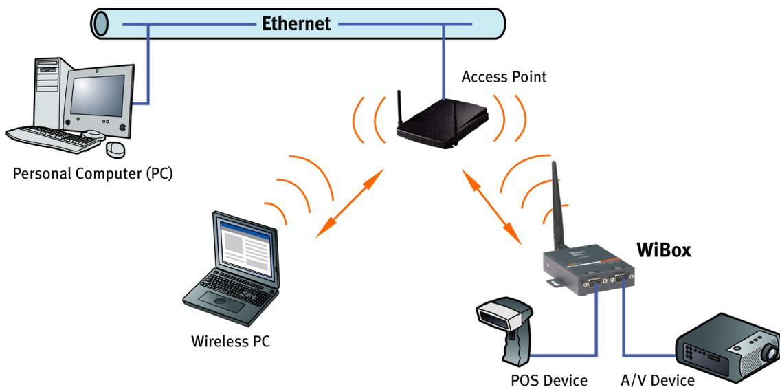
A PC connected to an AP via an Ethernet connection and a PC with a wireless connection to the AP LAN access the WiBox 2100E as though they are connected to it directly. The combination of the WiBox 2100E, a PC, and the Lantronix Redirector software allows the PC to communicate directly to the WiBox 2100E's serial devices, providing wireless serial tunneling.
