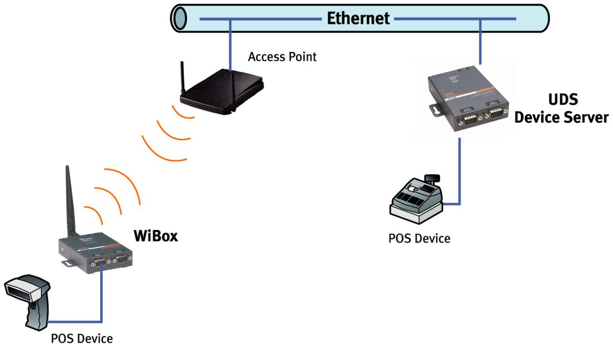
In the example above, the WiBox 2100E communicates with another device server via the AP. The WiBox device server, in this example, is connected via an Ethernet connection to the AP. In this way, the WiBox 2100E and the device server communicate directly and can transfer information between their serial devices.
