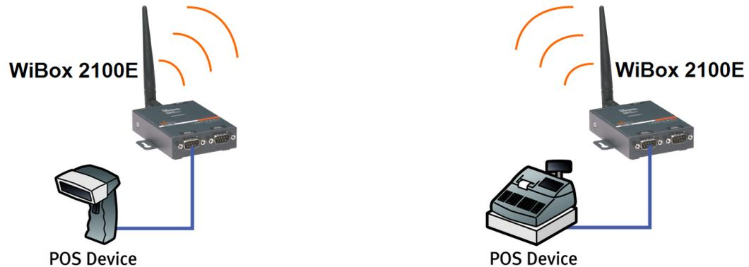
In the example above, the two WiBox 2100E devices have established an Ad Hoc peer-to-peer relationship. They communicate directly to each other's serial devices without a PC or an AP.
