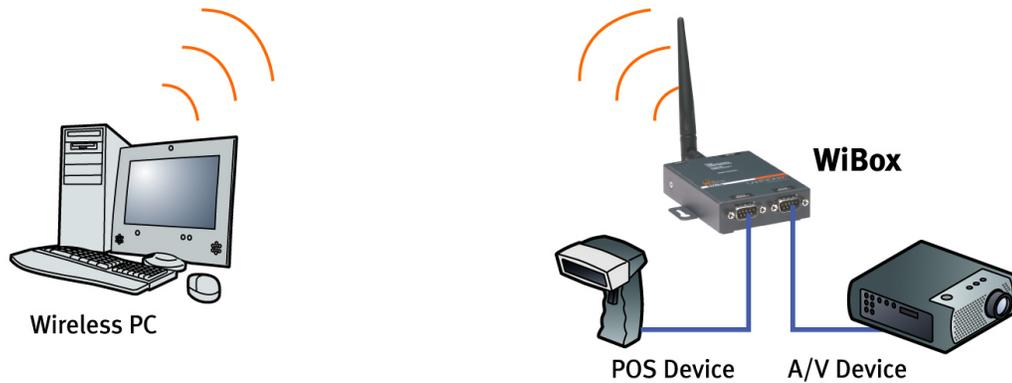
In the example above, the AP is not present. The PC makes a direct wireless connection with the WiBox 2100E to manage serial devices. Without an AP, it is a peer-to-peer relationship.
